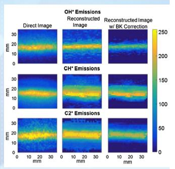
CO2 background-removed 2D OH, CH, and C<sub>2</sub> images of a Hencken flame at  $\phi$ = 1 using HSIS.
