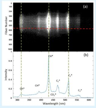
Spectrally and spatially resolved flame emission for premixed methane/air flame using HSIS. (a) Image recorded from spectrometer; (b) spectrum taken from Fiber No. 550 (spatial location is close to flame front).
